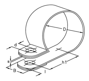
$\begin{array}{ll} d & = 6.4 \\ \text{Diameter D} = 12 \\ \text{h1} & = 15.7 \\ \text{I} & = 6.0 \\ \text{s} & = 0.6 \\ \text{Width B} & = 15 \\ \end{array}$
